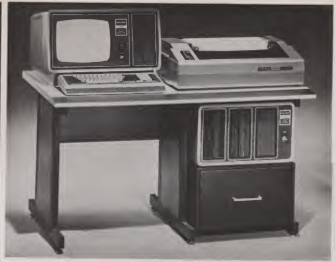
Model II microcomputer with line printer, external disk system and system desk.
